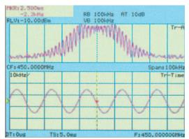
Spectrum and FM-demodulation waveform
